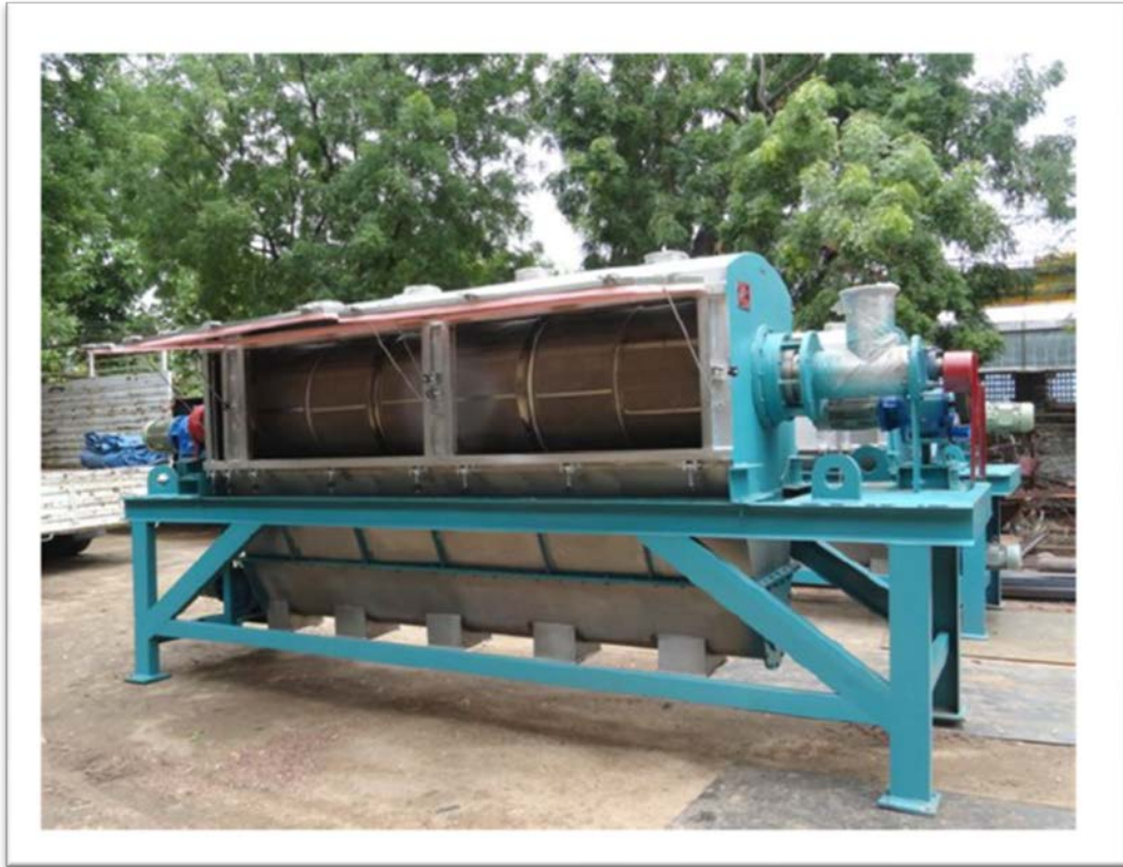
FINEX SR-6X ROTARY DRUM SIFTER OPEN VIEW IN STAINLESSTEEL 304
