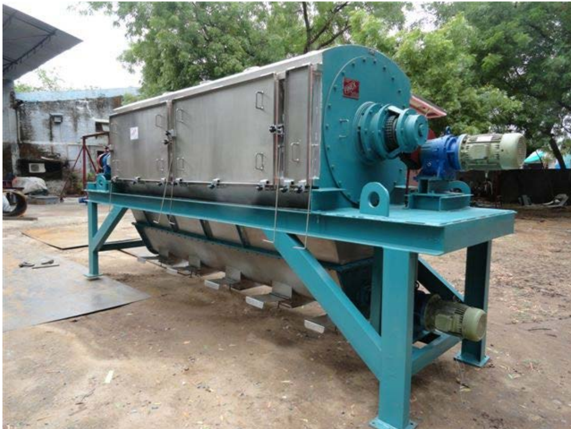
FINEX SR-6X ROTARY DRUM SIFTER CLOSED VIEW IN STAINLESSTEEL 304
