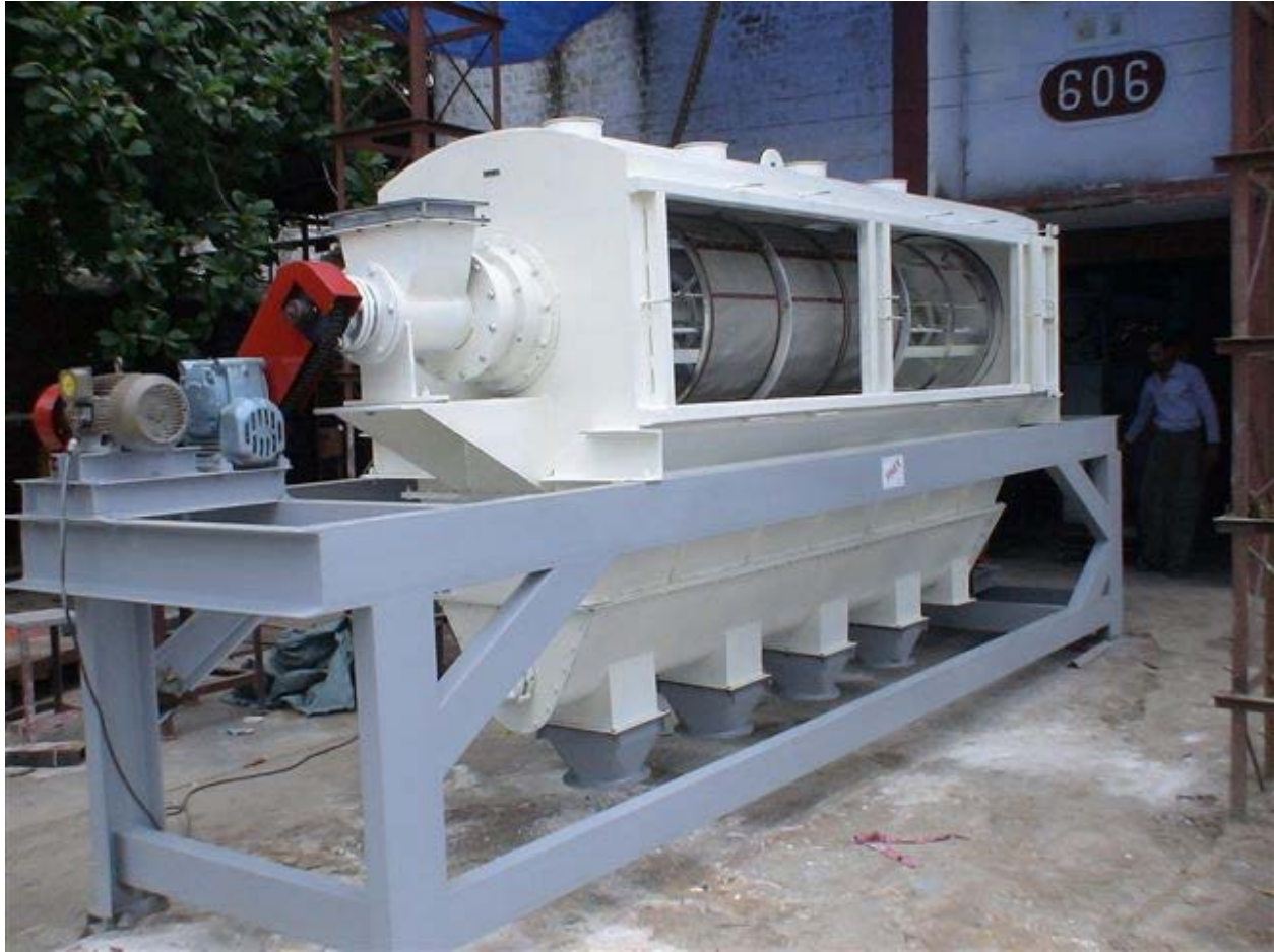
FINEX SR-6X ROTARY DRUM SIFTER OPEN VIEW IN MILD STEEL
