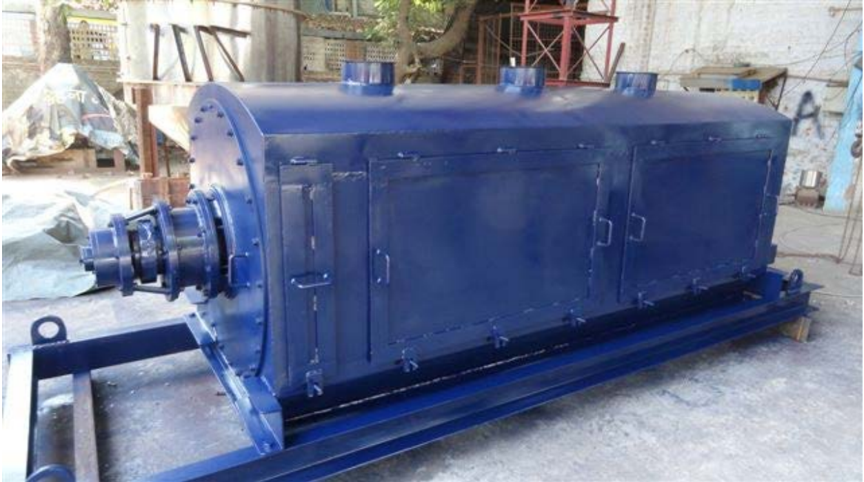
FINEX SR-5X ROTARY DRUM SIFTER CLOSED VIEW IN MILD STEEL
